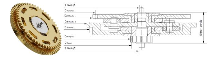
Our high-performance auxiliary reversing wheel guarantees maximum precision and reliability, especially due to the Feller-Roulage and the latest REACH-compliant materials. By applying the satellite principle, the 'Angle-Mort' is significantly reduced, resulting in a more efficient winding of the spring barrel.
