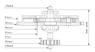
Our high-performance auxiliary reversing wheel guarantees maximum precision and reliability, especially due to the Feller-Roulage and the latest REACH-compliant materials. By applying the satellite principle, the 'Angle-Mort' is significantly reduced, resulting in a more efficient winding of the spring barrel.
